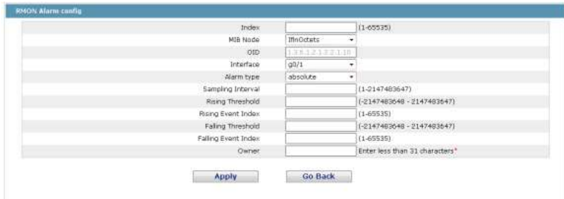
Figure 9-11: RMON Alarm Config
